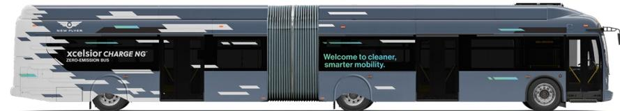
**New Flyer redesigned the 60-foot zero-emission, battery-electric Xcelsior CHARGE NG™ to include additional battery strings, increasing the range of the bus by ~30%**
