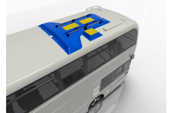
Byd Adl Enviro400ev With New Charging Options Roof Mounted Charging Rails
