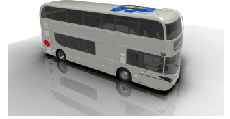
Byd Adl Enviro400ev With New Charging Options Roof Mounted Charging Rails
