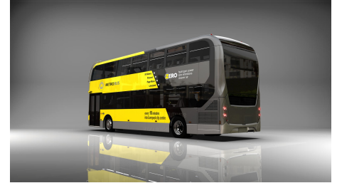
NFI zero-emission bus: the ADL Enviro400FCEV fuel cell electric bus for Liverpool City Region
