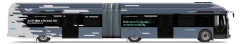
NFI - New Flyer Xcelsior CHARGE NG™ 60ft battery-electric zero-emission heavy-duty transit bus
